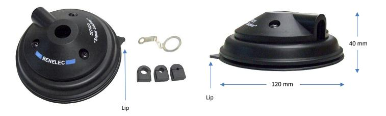
This universal Magnetic suction base provides the benefit of simple short-term installation of an antenna to any ferrous based metal panel. Ideally a vehicle panel will provide a suitable base for antenna mounting when a temporary installation is required. The base uses a combination of both air suction and magnetic force to secure the antenna to the vehicle. The only way to remove the base is to lift the lip of the suction cup to allow air to fill the vacuum created.
